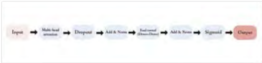
Fig. 3: Blocks of the transformer
