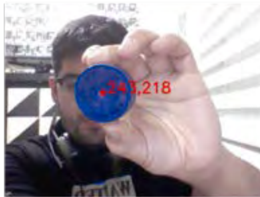
Figure 5. Real-time video capture and processing using OpenCV in Python. This system detects and tracks objects dynamically through HSV filtering and contour recognition
