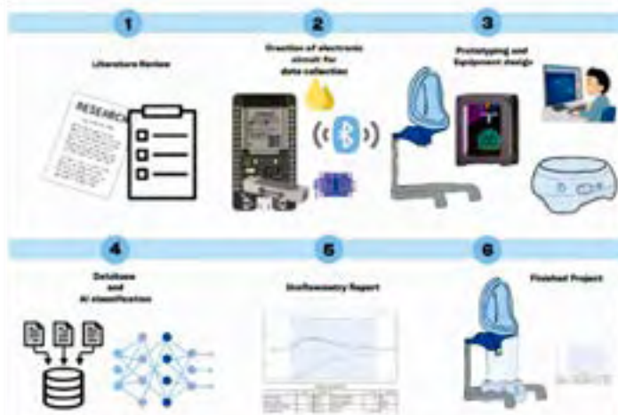
Fig. 1 Visual representation of the development flow of the FlowCare For U device, designed for the early detection of Lower Urinary Tract Symptoms (LUTS) from home. This process encompasses the review of literature to observe what has already been recorded, the creation of a low-cost circuit for data collection, the design of the prototype, the integration of AI for early diagnosis, and the completion of the device along with the patient's status report.
