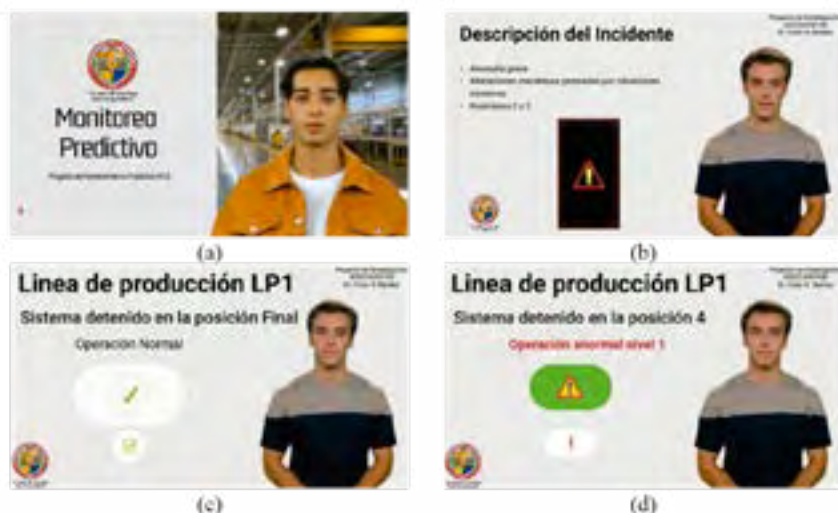
Fig. 4. Overview of the avatar-based fault reporting system. (a) A screenshot of the video corresponding to a daily summary report indicates that no failures occurred during the shift. (b) Screenshot reporting a fault event. (c) The screenshot indicates a normal operational state. (d) The screenshot reports an anomalous condition.
